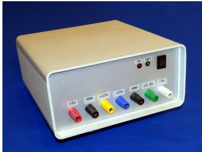
Figure 3 The author's ATX-based power unit makes a handy bench supply
